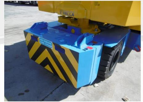
Removable ballasts to make it easier to transport the crane
